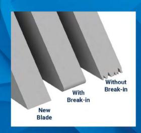
During the first cut, increase feed rate/force slightly once the blade fully enters the work piece.
