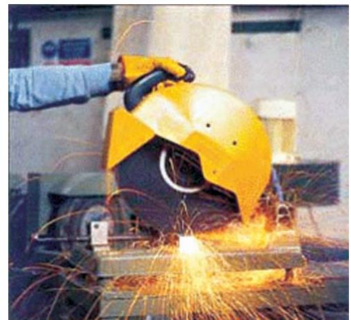
**USE BEFORE DATE:** On some DURA-KUT wheels, manufacturing date is stamped on the label. For example, 11021201-stamped means 11 (year) 02(month) 12(date) 01 (Machine number). The wheel is good for use upto 30 months from this date i.e. August 2013. On some wheels, the use-by year is pressed on the metal ring, like 2013 – meaning the wheel is good for use upto year 2013.
